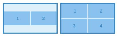
Multiview sources can be any combination of wired and wireless devices (Airplay & Miracast). For example, an iPad casting via AirPlay and a hardwired connection via HDMI can be in a split screen layout. Any combination is possible but limited to four simultaneous streams.
