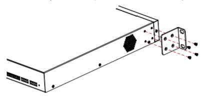
2. Screw the unit to the equipment rack (screws are not included in the package).
