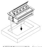
Once the hole has been cut to size, the product should simply slot into place. Make sure all cables are passed throught the hole first.
