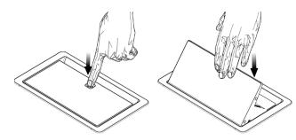
Open the product by simply pressing the button on the top of the flap. You can also open by just lifting up the flap. To close the unit, gently push the flap downwards until it clicks.
