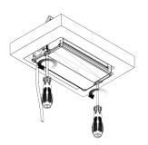
When the In-desk plate is situated in the hole, you can tighten the product in place by screwing the two Philips head screws at the bottom of the product.
