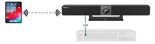
**AP Disabled**: This mode completely disables the built-in AP. This mode should be used when you plan to use an existing network's access point(s). This requires a LAN connection to the VX20 in order for it to be found and discoverable on the existing network.
