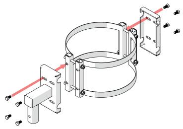
STEP 3 – Fix covers (loosely) to the Strap connecting bars with the  $4 \times M10 \times 25$  hex screws provided. Lift the whole unit to the desired height and tighten studding so that it clamps the straps to the pillar. Tighten cover screws. The VCC1 has an arm on one cover only. The VCC2 has arms on both covers.
