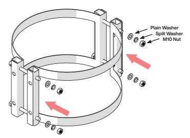
STEP 2 - Fix the studding together loosely using the plain and split washers and M10 nuts.
