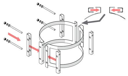
STEP 1 – Place both straps around your pillar, either on the floor or on a support. Place connecting bars into slots in straps and push the studding provided through the holes to attach them. NOTE: The open channel section of the bar must be positioned against the wall of the strap.
