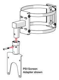
STEP 4 – Connect direct fitting adapter (ordered separately) to peg for screen or projector suspension. A through bolt (supplied with the adapter) must be used to connect the adapter to the peg. Take up any slack using the grub screws in the adapter socket.
