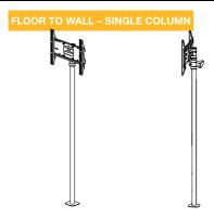
On Floor to Wall installations columns are 2m long. If necessary cut to desired height.
