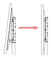
Using another team member, lift the screen up and gradually offer it up to the back plate. Gently tilting the screen forward, hook the arms over the rail of the back plate and lower into position.
