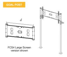
Goal Post columns are 2m long. If necessary cut to desired height. Identify the span-bar (screen size dependent), and measure the socket centre-to-centre distance (d).
