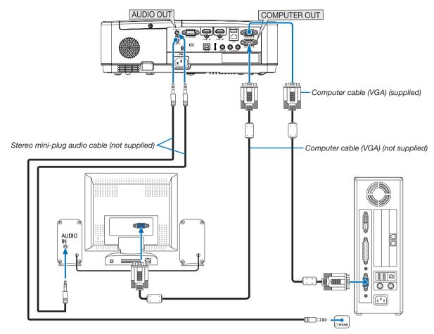
You can connect a separate, external monitor to your projector to simultaneously view on a monitor the computer analog image you're projecting.
