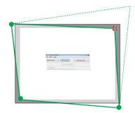
5. Repeat Step 3 and 4 to correct the distortion of the projected image.
