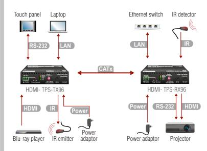
Connect the TPS output port of the Transmitter to the TPS input port of the CATx Receiver by a CATx cable.
