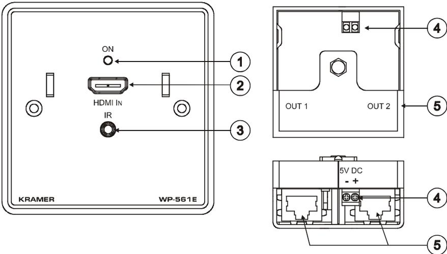
Figure 2: WP-561 HDMI Line Transmitter UK/European Model Functions
