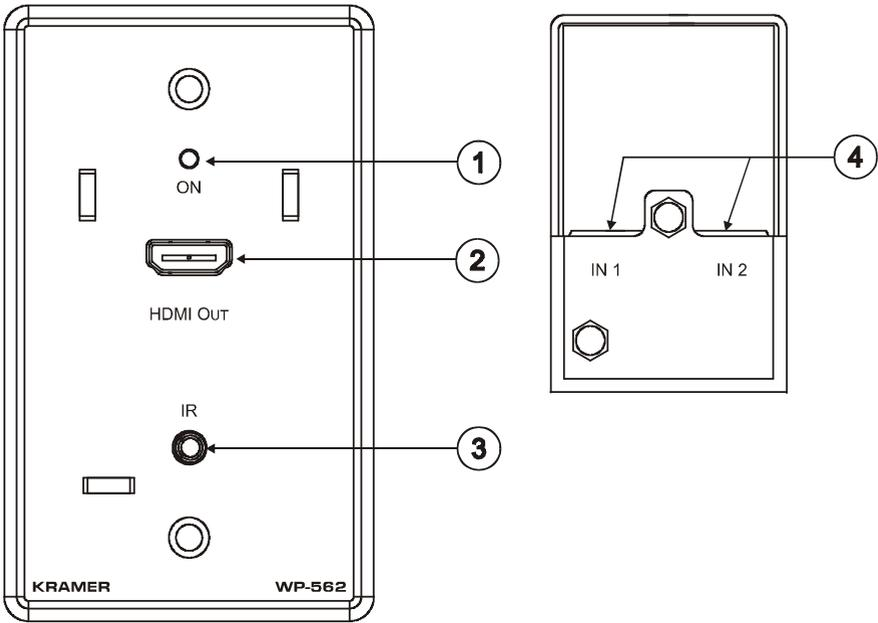
Figure 6: WP-562 HDMI Line Receiver US Model Functions
