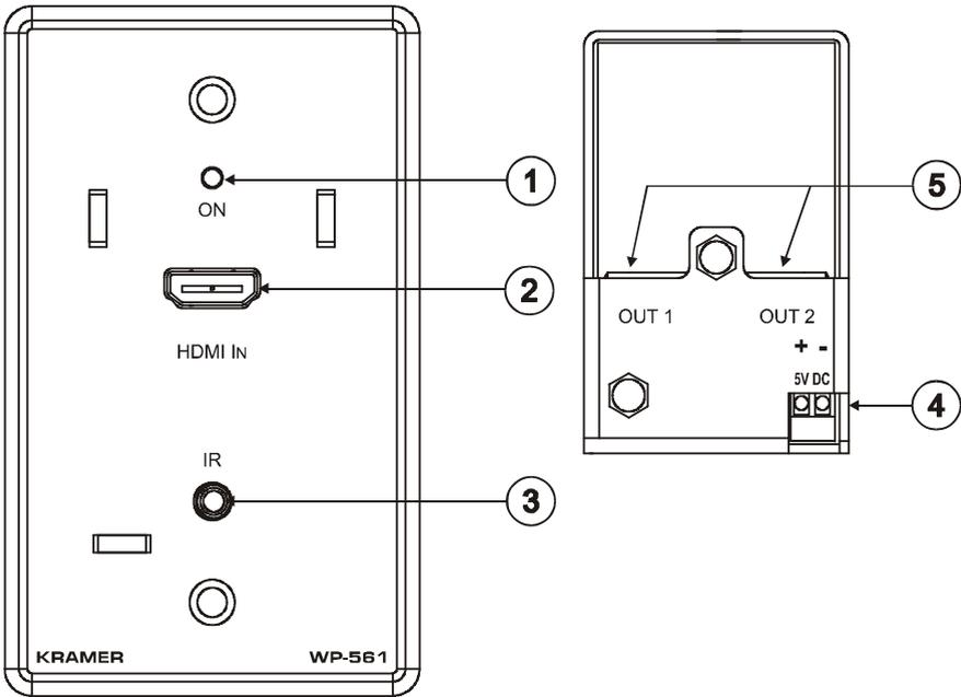
Figure 3: WP-561 HDMI Line Transmitter US Model Functions
