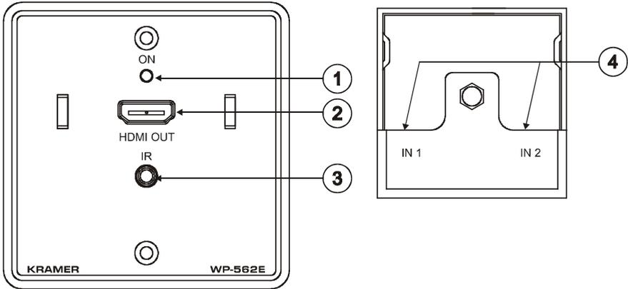
Figure 4: WP-562 HDMI Line Receiver Belgian/German Model Functions
