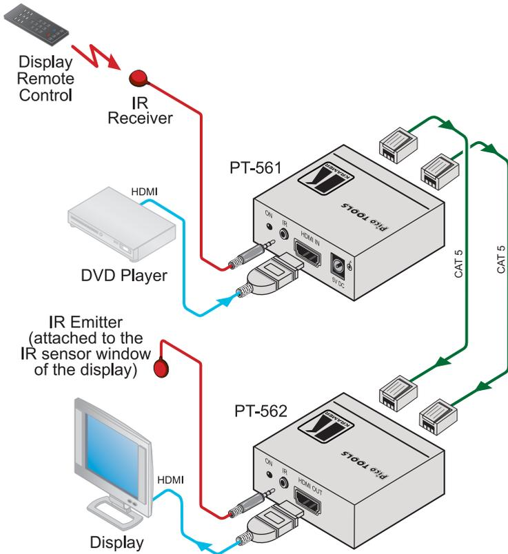
Figure 9: Connecting the PT-561/PT-562 HDMI Line Transmitter/Receiver
