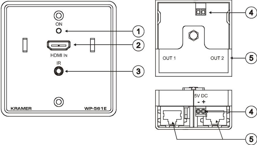
Figure 1: WP-561 HDMI Line Transmitter Belgian/German Model Functions
