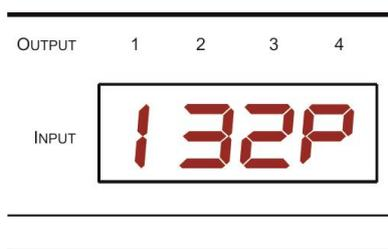
In this example: Input 1 is routed to output 1, input 3 is routed to output 2, input 2 is routed to output 3 and a pattern is routed to output 4.
