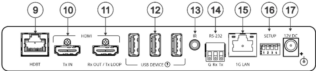
Figure 3: TP-600TRxr 4K60 HDMI/USB Extender Rear Panel
