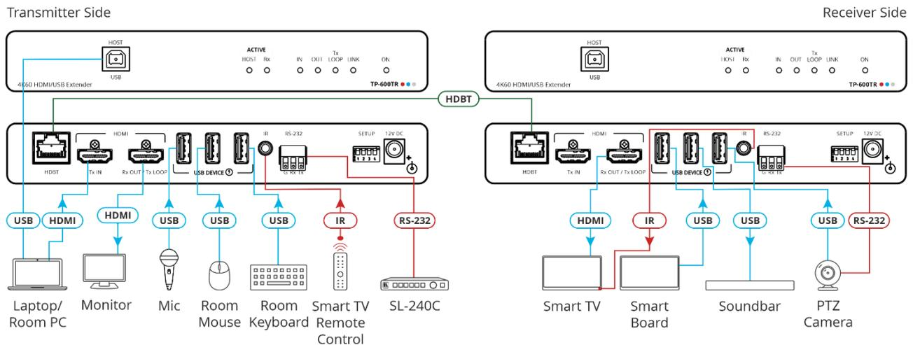
Figure 6: Connecting to TP-600TR
