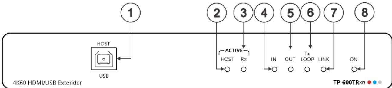
Figure 1: TP-600TRxr 4K60 HDMI/USB Extender Front Panel
