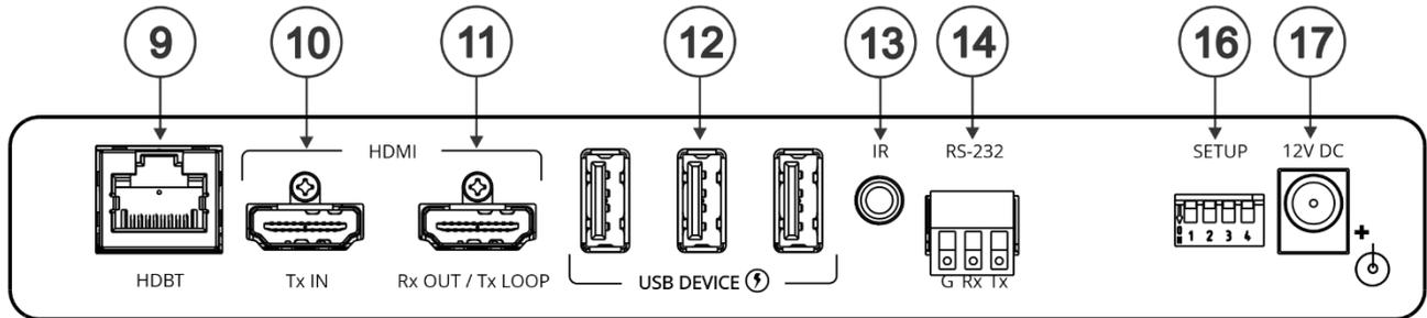
Figure 4: TP-600TR 4K60 HDMI/USB Extender Rear Panel
