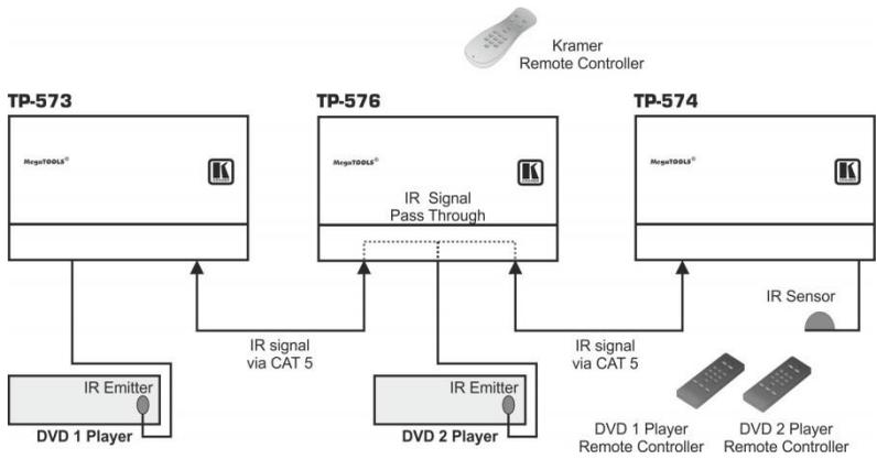
Figure 6: TP-576 IR Control – Example III
