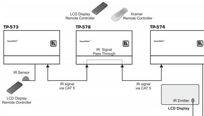
Figure 5: TP-576 IR Control – Example II
