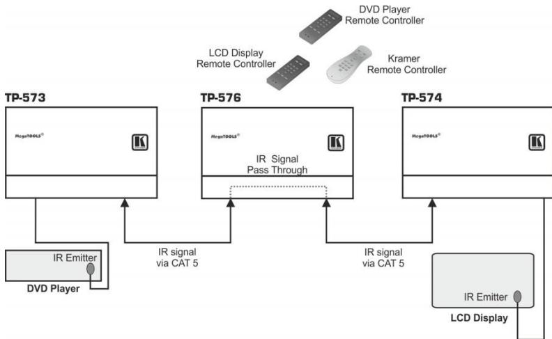
Figure 4: TP-576 IR Control – Example I
