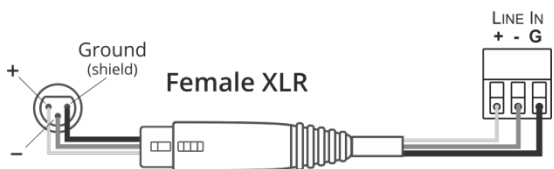
Figure 3: Connecting a Balanced XLR Input
