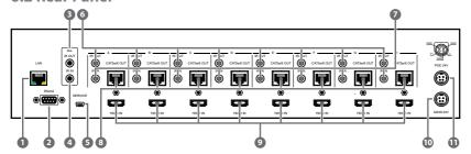
**LAN:** Connect to an active network for LAN serving and Telnet and Web GUI control (refer to Sections 6.8 and 6.9).
