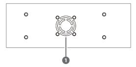
**1 Fan Ventilator:** These are air ventilation areas, DO NOT block these areas or cover with any object. Please allow adequate space around the unit for air to circulate.
