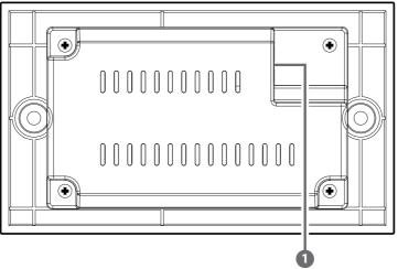
**CAT OUT:** Connect to the Receiver unit with a single CAT5e/6/7 cable for transmission of all data signals.
