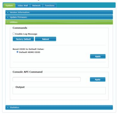
Finally, individual Telnet commands may be sent to the unit by using the "Console API Command" text entry field and pressing "Apply". Any responses from the unit will be displayed in the "Output" field.
