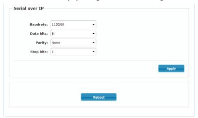
■ **Serial Settings:** Set the desired baud rate, data bits, parity, and stop bit for the RS-232 signal to extend.
