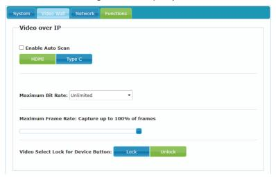
■ **Source Selection:** Select the preferred input source, HDMI or Type-C or enable the auto scan function of the unit by checking the "Enable Auto Scan" checkbox.
