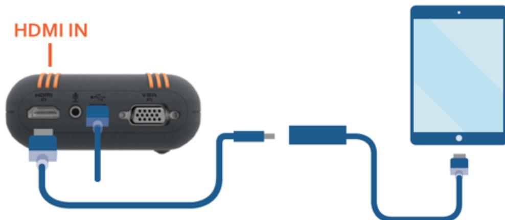
Figure 9: Connecting to a smartphone/tablet using HDMI
