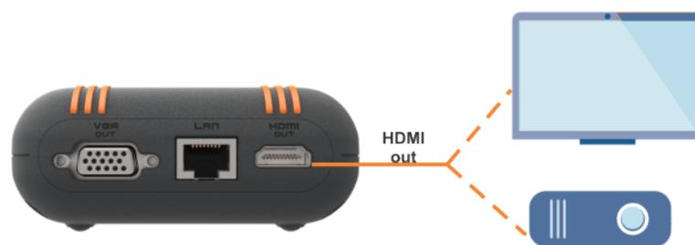
Figure 12: Connect to a room display using HDMI
