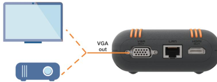
Figure 13: Connect to a room display using VGA
