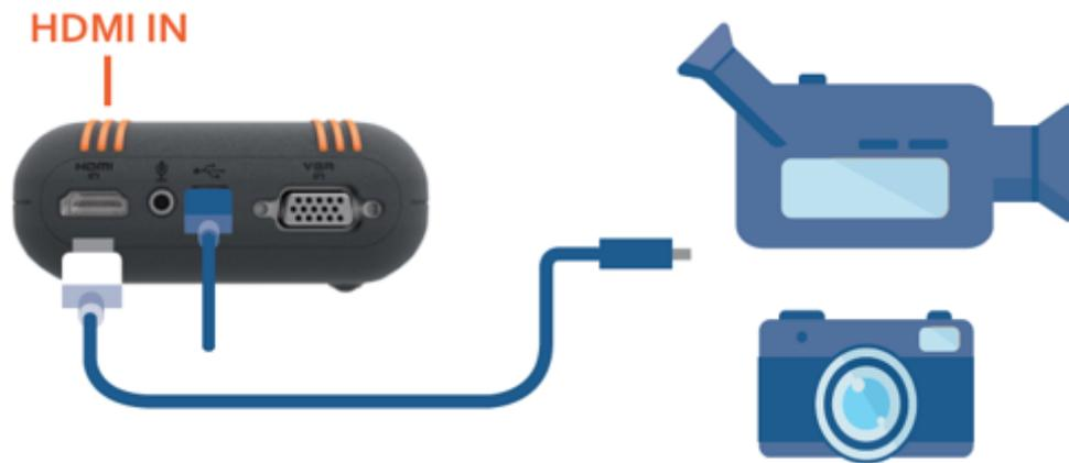
Figure 11: Connecting to a digital camera with HDMI
