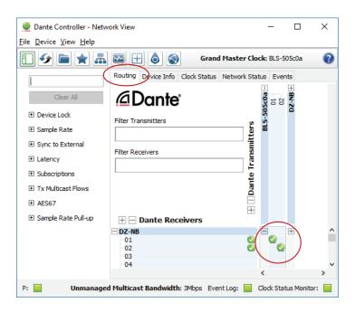
By default the DA11ADE is shipped with its network settings set to obtain an IP Address automatically. This means that if a DHCP server is present on your network, it will provide the DA11ADE with an IP Address. If no DHCP server is present then the DA11ADE will receive a default IP Address in the 169.254.xxx.xxx range. To change the IP Address of the DA11ADE, you must enter the "Network Config" menu in the "Device Info" screen of the Dante Controller software.
