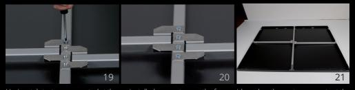
Horizontal struts are mounted at the preinstalled connectors on the frame side and on the center supports at the M6 thread inserts with countersunk screws.
