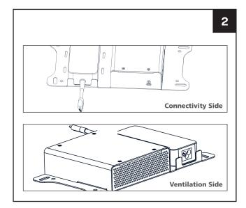
Check the orientation of the PSU. Power-In socket towards ventilation side of BX.
