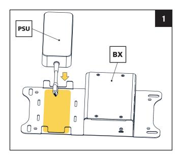
Attach the PSU to the BX mounting plate with cable ties or bands
